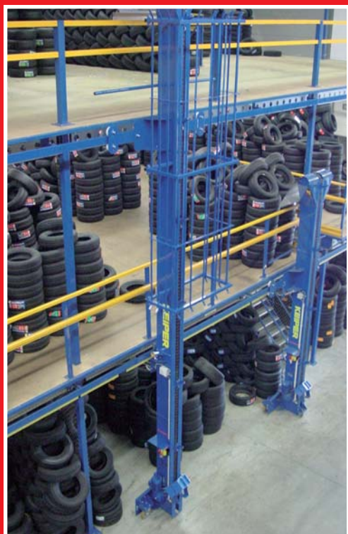
Mobile tyre elevator in a tyre warehouse feeding various warehouse levels.
