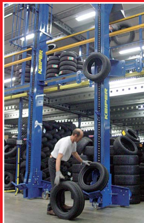
Mobile tyre elevators, manually movable, for conveying heights between 4 and 8 m, in a large tyre-depot.
